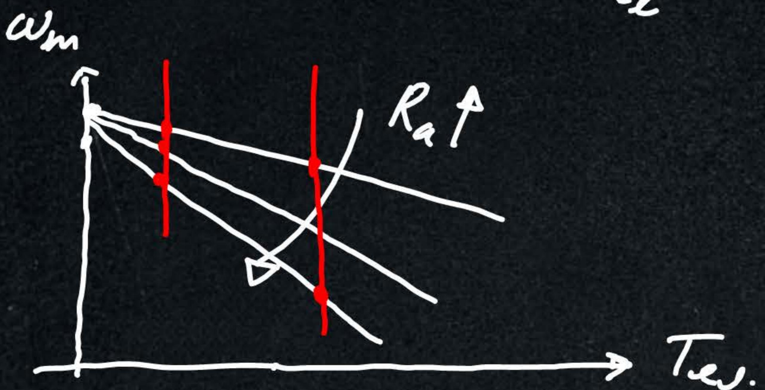
Torque-speed equation (series DC motor)
